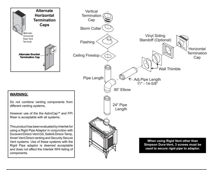
The FPI AstroCap<sup>™</sup> and FPI Riser Vent terminal are certified for installations using FPI venting systems as well as Simpson Dura-Vent<sup>®</sup> Direct Vent GS, American Metal Products Ameri Vent Direct Vent, Security Secure Vent<sup>®</sup>, Selkirk Direct-Temp. AstroCap<sup>™</sup> is a proprietary trademark of FPI Fireplace Products International Ltd. Dura-Vent<sup>®</sup> and Direct Vent GS are registered and/or proprietary trademarks of Simpson Dura-Vent Co. Inc.
